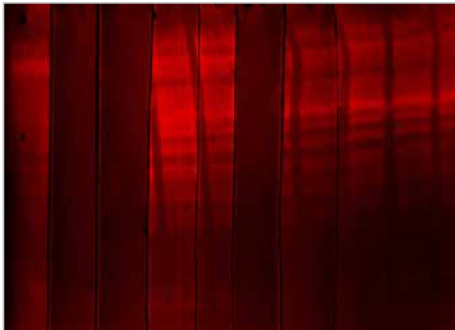
Dy-Light 635 labeled antibodies on PVDF-Western Blot membrane, detected by excitation with 625nm LEDs and 680nm emission filter. Color applied afterwards.
