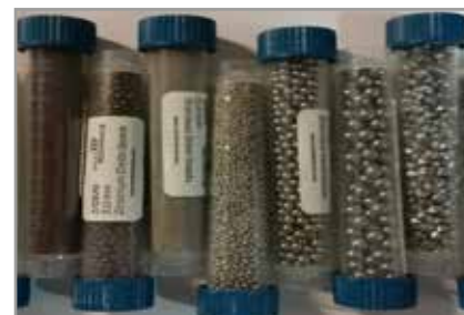
Different beads (stainless steel, glass, zirconium oxide, zirconium silicate)
